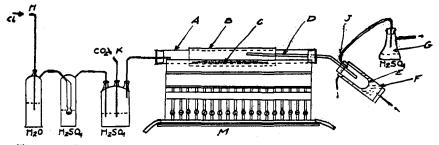
The reaction tube A, is made of hard glass about 5 cm. in diameter and about 150 cm. long. A sheet iron jacket, B, 8 cm. in diameter, surrounds this tube and leaves an air space of about 1 cm. between it and the glass. This permits of a uniform and slow heating of the tube—the heat being easily regulated by the combustion furnace, M. The ferro-vanadium is crushed to about 4 mesh and placed in the reaction tube at C. An inclined delivery tube, D, extends into the receiver E, which is sur-
